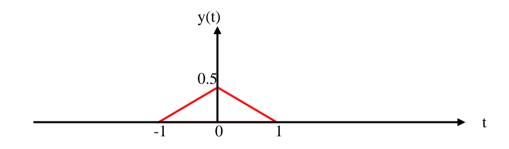
➤ Amplitude scaling form of given triangular signal is
