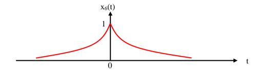
Given  $x_6(t)$  is bounded signal, because its amplitude is finite for all values of t (limited to 0 and 1)
