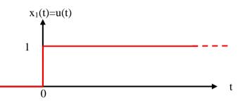
Given  $x_1(t)$  is bounded signal, because its amplitude is finite for all values of t (limited to 0 and 1)
