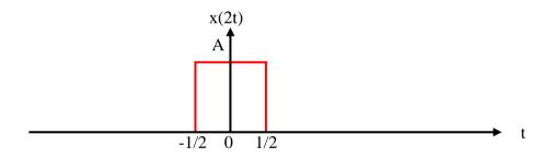
$\triangleright$  Time Scaling (Expanded) form of x(t),
