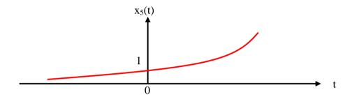
Given  $x_5(t)$  is unbounded signal, because its amplitude is infinity at  $t = \infty$ .
