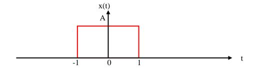
$\triangleright$  Time Scaling (Compressed) form of x(t),
