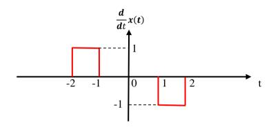
$$\frac{d^{2}}{dt^{2}}x(t) = \frac{d}{dt}\left(\frac{d}{dt}x(t)\right) = \frac{d}{dt}u(t+2) - \frac{d}{dt}u(t+1) - \left(\frac{d}{dt}u(t-1) - \frac{d}{dt}u(t-2)\right)$$
