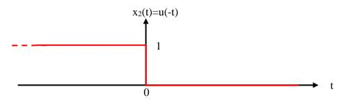
Given  $x_2(t)$  is anti-causal or non-causal signal, because it is left sided (Extending from  $t=-\infty$  to 0)
