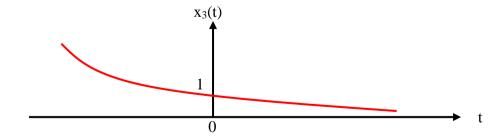
Given  $x_3(t)$  is unbounded signal, because its amplitude is infinity at  $t = -\infty$ .
