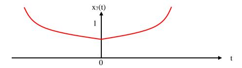
Given  $x_7(t)$  is unbounded signal, because its amplitude is infinity at  $t = \pm \infty$ .
