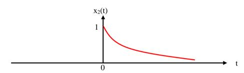
Given  $x_2(t)$  is bounded signal, because its amplitude is finite for all values of t (limited to 0 and 1)
