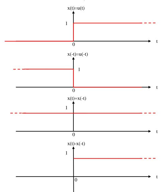
$x(-t) \neq x(t) \Rightarrow$  Given signal is not an even signal &
