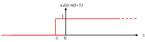
Given  $x_4(t)$  is non-causal signal, because it is both sided (Extending from t=-1 to  $\infty$ )
