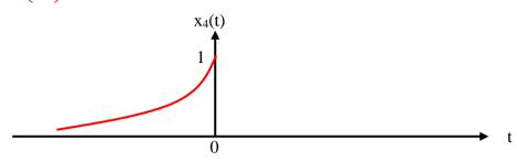
Given  $x_4(t)$  is bounded signal, because its amplitude is finite for all values of t (limited to 0 and 1)
