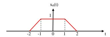
Given  $x_6(t)$  is non-causal signal, because it is both sided (Extending from t=-2 to 2)
