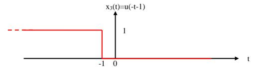
Given  $x_3(t)$  is anti-causal or non-causal signal, because it is left sided (Extending from  $t=-\infty$  to -1)
