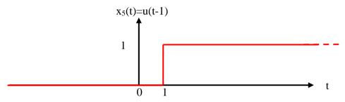
Given  $x_5(t)$  is causal signal, because it is right sided (Extending from t=1 to  $\infty$ )
