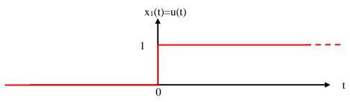
Given  $x_1(t)$  is causal signal, because it is right sided (Extending from t=0 to  $\infty$ )
